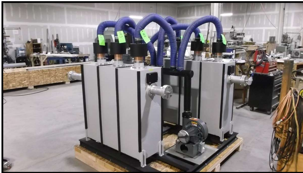
Shown above is Micronetixx Communications' High-Power FM Transmitter Diplexer
